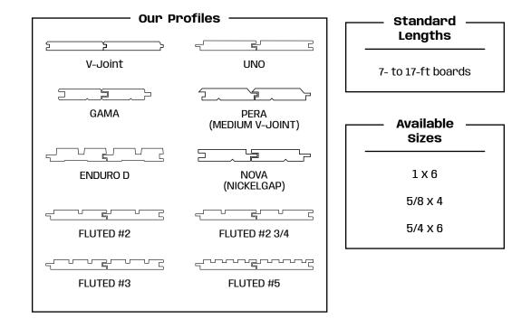
Thermowood® is manufactured using the metric system, which means that a foot-long measurement is always under 12 inches.
